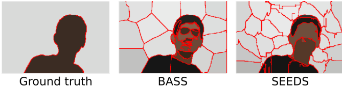
Figure 4: Two segmentations with similar UE (BASS: 0.0077, SEEDS: 0.0112). The segmentation with BASS (with a VOI of 2.5340, lower than the value for SEEDS 2.8095) contains the same information with less superpixels.
